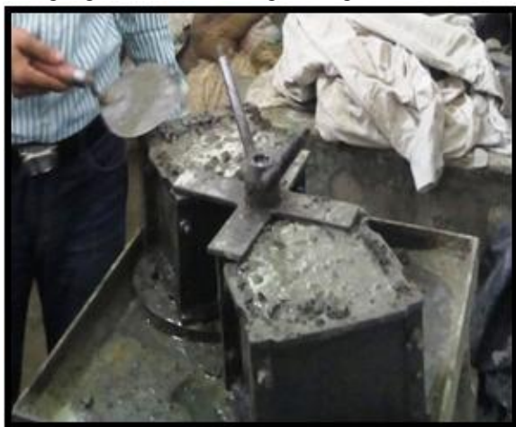
Figure 2. Compaction of concrete. (vibration)
