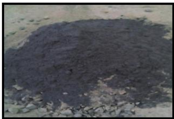
Figure 1. Coconut fibre ash mix in concrete proportion.
